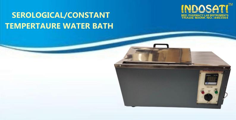
This unit are double walled with inner chamber made up of stainless steel and outside of mild steel duly enamel painted. The gap between the walls is fitted with special grade glass wool in order to avoid thermal losses. The inner chamber fitted with immersion type heating element is covered with perforated removable diffuser tray. Top cover is provided with the unit as a standard accessory.
