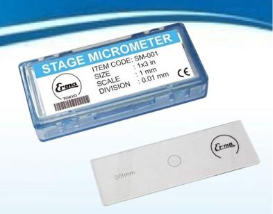
Stage Micrometer Accurately measures specimen under the microscope with scales attched in a glass microscope slide. The 1mm scale is divided to 100 accurate parts and comes in a standard 1" x 3 " slide protected by cover slip.
