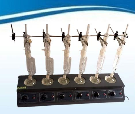
Soxhlet Extration Unit for 100 to 500 ml flasks with one energy regulator for controlling all baths individual ON/OFF switches with glass parts. Two adjustable rods with clamps.
