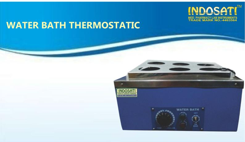
It is double walled with inner chamber made of stainless steel and outer wall of M.S sheet duly enamel painted. The gap between outer and inner walls is fitted with special grade glass wool insulation. The concentrate rings can be removed to accommodate containers of various sizes.
