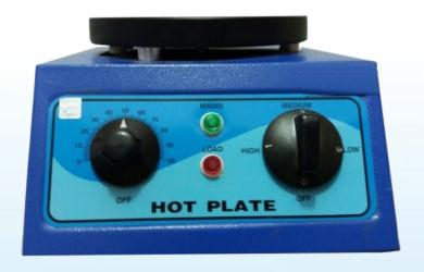
Hot Plate Round mounted on a thick **M.S. sheet body**, a smooth surface **cast iron plate** fitted with an electrically operated element laid under the plate. A three step rotary switch work on 220/230 volts A.C controls heating The plate is finished in heat resistant black and the body in stove blue white.
