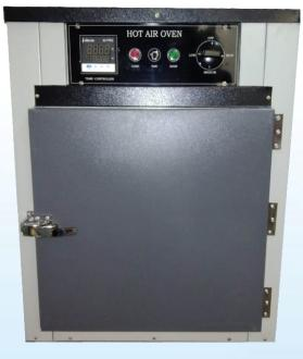
These are sturdy double walled units with outer chamber made of MS sheet duly enamel painted with inner made up of anodized aluminum or high SS sheet. The gap between inner and outer chamber is filled with high grade glass wool to avoid thermal looses. Heating elements are placed in ribs ,at bottom and sides .Inner chamber is provided with ribs for adjusting perforated shelves to convenient height. The
