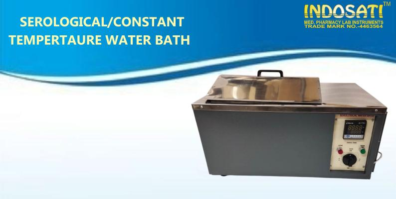
This unit are double walled with inner chamber made up of stainless steel and outside of mild steel duly enamel painted. The gap between the walls is fitted with special grade glass wool in order to avoid thermal losses. The inner chamber fitted with immersion type heating element is covered with perforated removable diffuser tray. Top cover is provided with the unit as a standard accessory.
