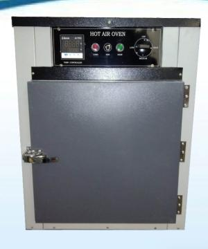
These are sturdy double walled units with outer chamber made of MS sheet duly enamel painted with inner made up of anodized aluminum or high SS sheet. The gap between inner and outer chamber is filled with high grade glass wool to avoid thermal looses. Heating elements are placed in ribs ,at bottom and sides .Inner chamber is provided with ribs for adjusting perforated shelves to convenient height. The
