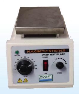
It has a compact stirring device utilization a rotating magnetic field (created by a PERMANENT MAGNET) which induces variable speed stirring action. Stirring is accomplished by means of small TEFLON rotor, which when placed in the liquid to be stirred is capable of rotation by magnetic field applied from below the container. The unit is fitted with pilot lamp. To work on 2220/230 volts A.C. available with or without hot plate (as required).
