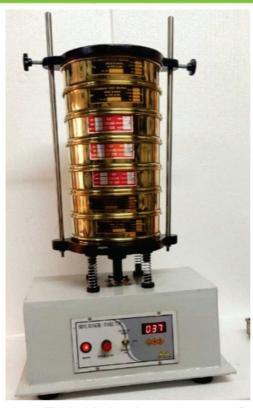
we are presenting for our clients a vast range of Sieve Shaker - Table Model. As per the specific clients' requirements, this shaker is available with FHP electric motor inside the body. Apart from this, adroit professionals use quality proven components and the latest technology in line with industry norms. Speed can be regulated in this shaker through an unceasingly variable speed regulator placed to the unit.
