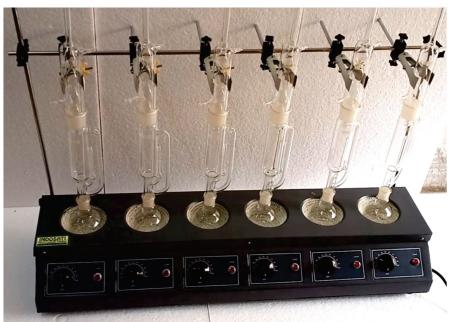
Bath type for 100 to 350 ml flasks with one energy regulator for controlling all baths individual ON/OFF switches without glass parts. Two adjustable rods with clamps.
