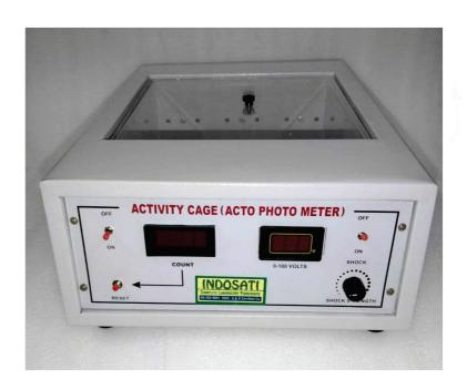
The Digital Actophotometer provided by us consist of six built in photo sensor and four digital counters to indicate the loco meter activity. Our Digital Actophotometer measures the spontaneous and indicated activity with digital totalizes. It also incorporates electric shock of upto 100volts for activating rats. Our Digital Actophotometer can measure stimulus of is variable from 0-100volt and indicating on meter.
