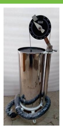
Spirometer mainly used as Gasometers in the Research Labs, Medical institutions and many other Labs. These are featured with the 6 liter of vital capacity; with chain compensate counter balance to float through pulley, calibrator to denote volume, inlet, & outlet tubes, stainless steel chamber; complete with corrugated rubber tubes. For the manufacturing and supplying of these Spirometers, we have positioned an apex.
