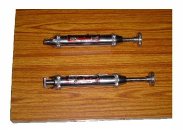
A fairly handy instruments for taking quick readings for the hardness of tablets. It is made of brass turned parts, heavily chrome plated, the scale is 0 to 20 kg and the index mark and division is in 1 kg reading. Scale adjustable for zero setting as per size of the tablets.
