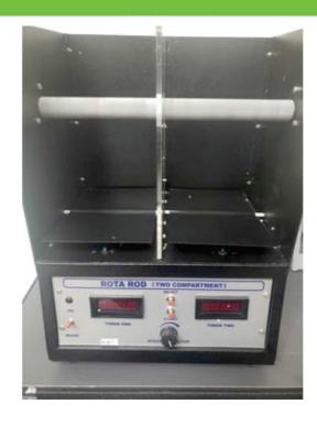
The Rotarod Apparatus provided by us come with latest with digital counter, for determining neuro-pixicity, muscle tone, balance and motor co-ordination in rats and mice. Our Rotarod Apparatus have two or three or four compartments of 75mm width each with a rotating rod of 25mm diameter having speeds of 5,10,15,20 and 25 r.p.m with time interval countries in each compartment.
