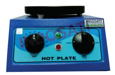
Mounted on a thick M.S. sheet body, a smooth surface cast iron plate fitted with an electrically operated element laid under the plate. A three step rotary switch works on 220/230 volts A.C. controls heating. The plate is finished in heat resistant black and the body in stoved blue white.
