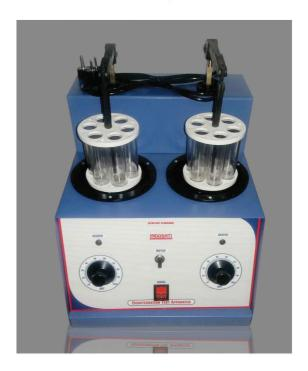
Our Disintegration Testing Machine is fitted with a motorized shaft moves in and up and down direction at a frequency of 30 cycles per minute. It can hold 6 glass tubes of standard size with stainless steel wire gauge bottom. Our Disintegration Testing Machine has a cylinder which can moves up & down with standard dish inside in a 1Ltr.Beaker filled with distilled water which is maintained at 30oc by thermostatically controlled hot plates(without beaker)
