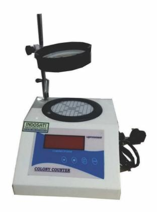
An ideal instrument for counting bacterial mould colonies in culture work. It provides uniform glare free illumination to minimize strain on eyes and clearly define even small colonies. A 100 mm dia lens covers the entire illumination field and its magnification assures highly accurate results. Counting plate with standard Wolfhugel ruling ensures clearly differentiated and sharply defined colonies. Supplied complete with counting plate, lens, cord and plug. To work on 220VAC supply.
