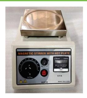
It has a compact stirring device utilization a rotating magnetic field (created by a PERMANENT MAGNET) which induces variable speed stirring action. Stirring is accomplished by means of small TEFLON rotor, which when placed in the liquid to be stirred is capable of rotation by magnetic field applied from below the container. The unit is fitted with pilot lamp. To work on 220/230 volts A.C. available with or without hot plate (as required).
