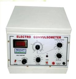
The Electro- Convulsiometer is the instrument used for applying maximal Electro shock through the corneal electrodes provided with the instrument. It is used to study the anti-convulsant activity of phonation against maximal electro shock induced convulsions in rats.
